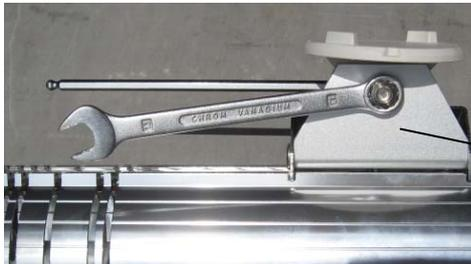
Fasten coupling flange to the heat transmission unit.
