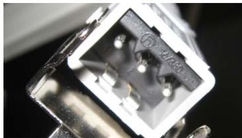
Mount the plug half with the open contacts (STAS3) on the side of the heat transmission unit.
