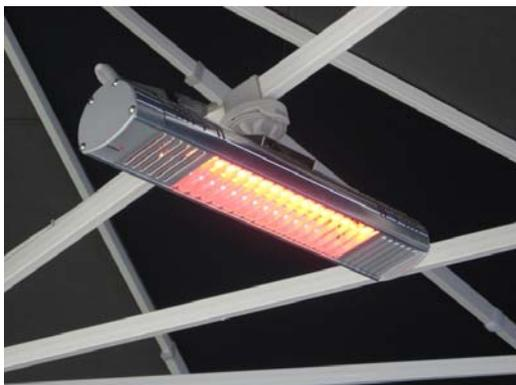
Before switching on the heat transmission unit, rotate it into a horizontal position, otherwise the service life of the heating tube will be reduced.
