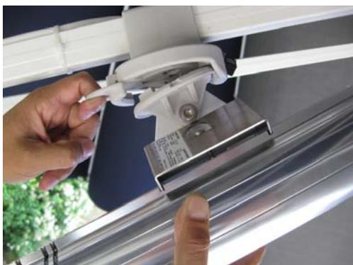
Hold the heat transmission unit with one hand and pull the operating ring of the quick-fit coupling with the other hand. With the operating ring pulled, pivot the coupling flange from the quick-fit coupling and remove the heat transmission unit.
