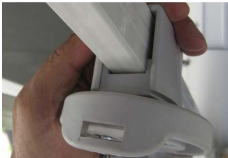
Fasten quick-fit coupling to the sunshade frame where suitable. For an installation on reinforced rods, remove the insert. Insert heat transmission unit (with coupling flange) into the quick-fit coupling (see 6.1)
