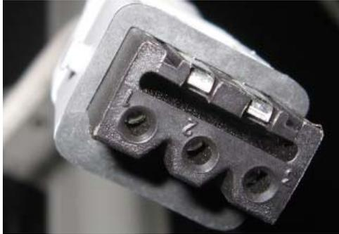
Mount the plug half containing the screen-protected contacts (STAK3) on the live side.
